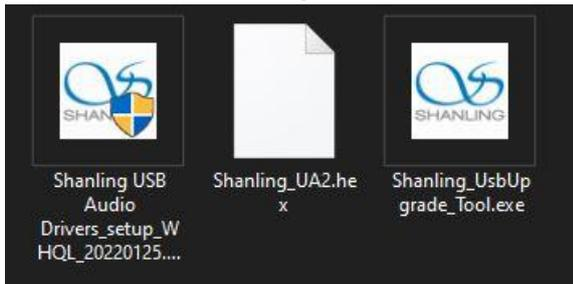
2. Open the “Shanling USB Audio Drivers\_setup” to install the latest UA model USB Drivers. You might be asked to uninstall older drivers and restart your computer before the installation can start. You will be asked to connect the UA model during driver installation.
