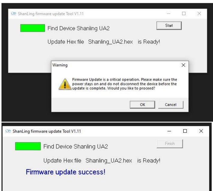
6. When finished, disconnect the UA model. Firmware Update is done.
